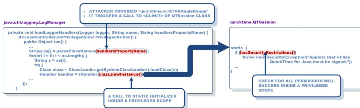
**ORACLE'S ISSUE 15 IS ABOUT LOADCLASS / NEW INSTANCE INSIDE DOPRIVILEGED BLOCK (BYPASS OF <CLINIT> SECURITY CHECKS)**
